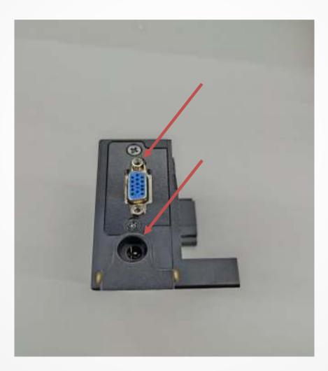
5. Please remove the holder of the hardware boards by unscrewing the 4 screws.
