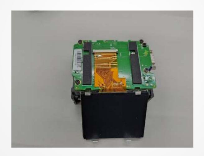
8. Please remove the LCD board from the main board by carefully unplugging the golden pins.
